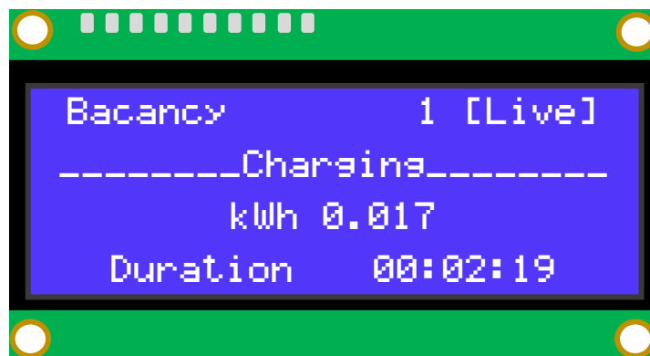
Figure 6 Energy Consumption and Time Duration in Charging Mode.
