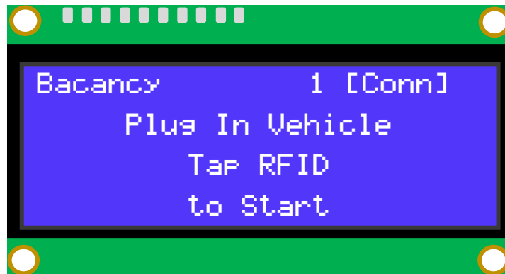
Figure 4 To Start Charging, Plug-in Vehicle and Tap the RFID.
