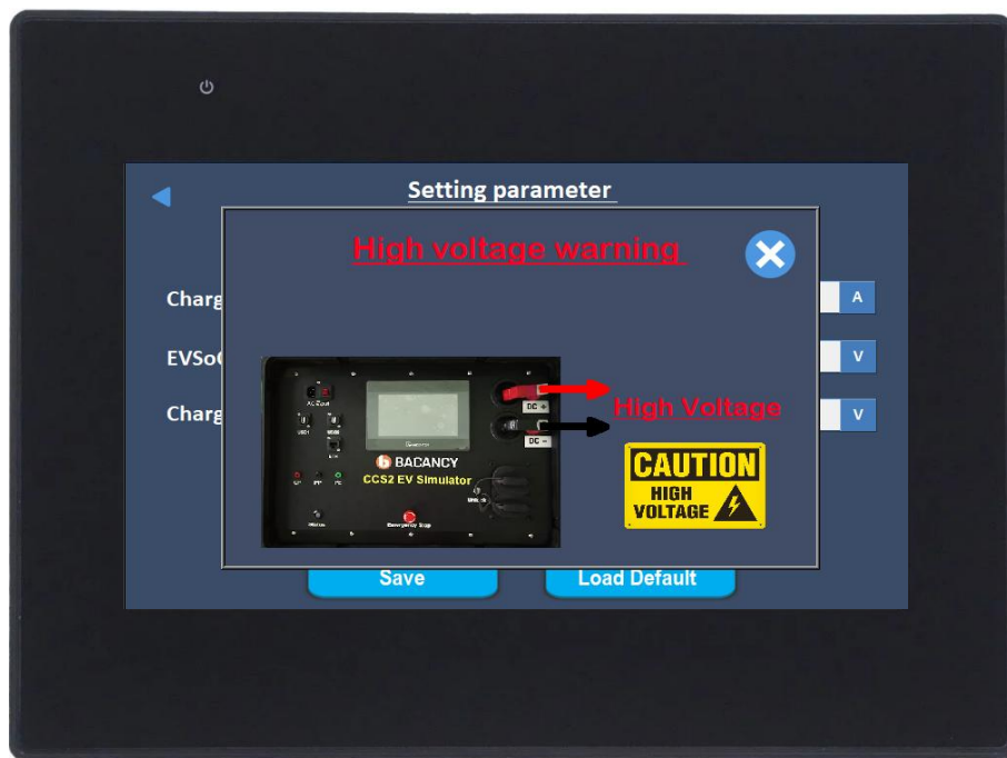
Figure 7 High Voltage Warning on Screen
