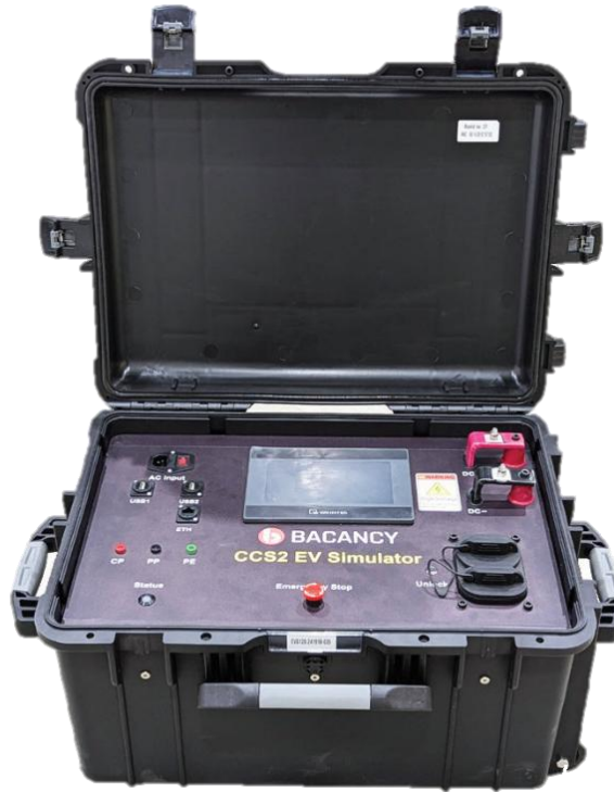
Figure 2 CCS2 EV Simulator (120 kW)
