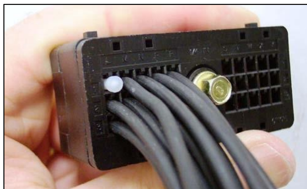
Figure 16 wires in the outer rows.
