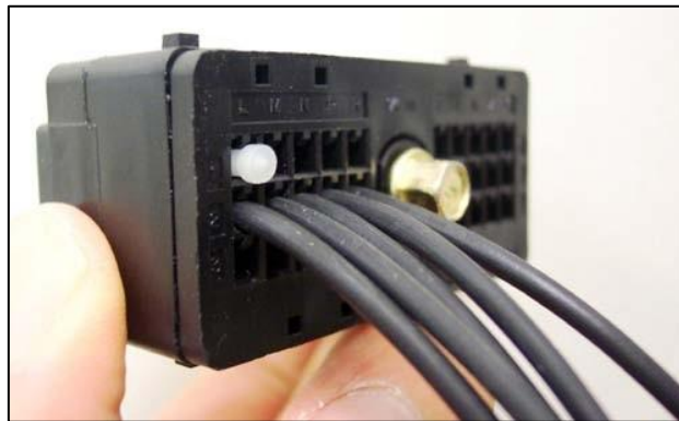
Figure 15 Wires in the middle row.
